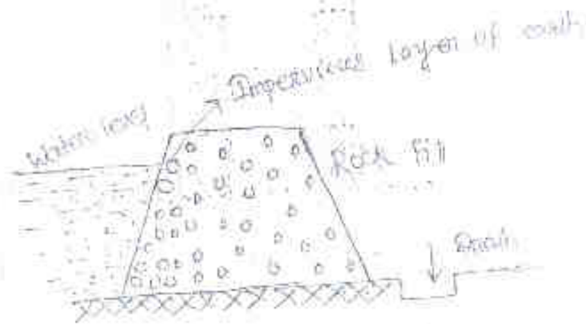
Rock fill coffee dam
