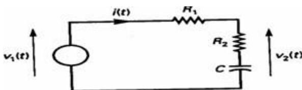
$$R_1 i(t) + R_2 i(t) + \frac{1}{C} \int_0^t i(t) dt = v_1(t)$$
