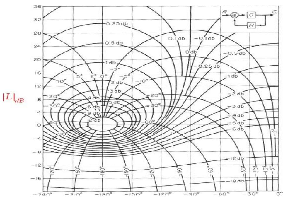
And  $|L(j\omega)$  which corresponds to a constant  $\alpha(j\omega)$  can be drawn as a locus of M circle on this plane as shown below
