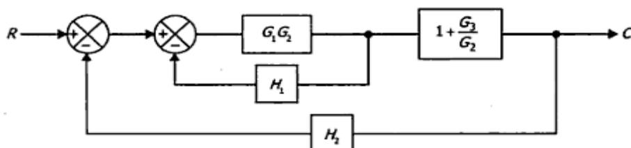
Replacing the internal feedback loop
