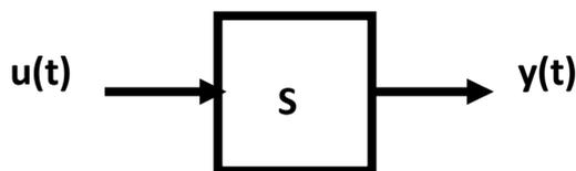
$$\frac{d^n y}{dt^n} + a_{n-1} \frac{d^{n-1} y}{dt^{n-1}} + \dots + a_0 y(t) = b_{m-1} \frac{d^{m-1} u}{dt^{m-1}} + \dots + b_0 u(t)$$
