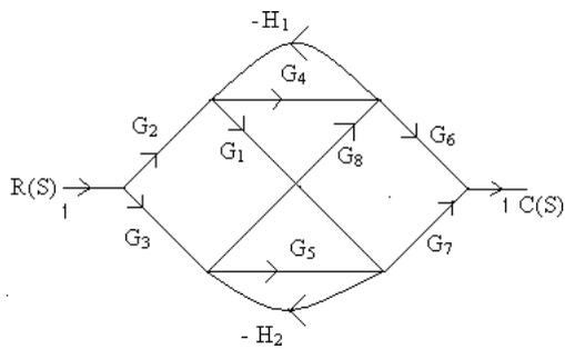
7. Draw a signal flow graph and evaluate the closed loop transfer function of a system Whose block is shown in fig?
