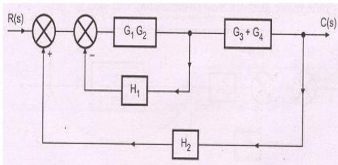
Reduce minor feedback loop of  $G_1, G_2$  and  $H_1$
