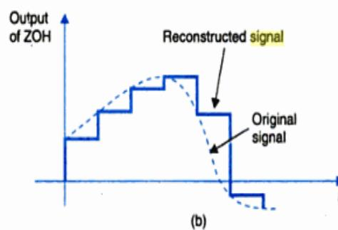
The high frequency noises present in the reconstructed signal are automatically filtered out by the control system component which behaves like low pass filters. In a first order hold the last two signals for the current sampling period. Similarly higher order hold circuit can be devised. First or higher order hold circuits offer no particular advantage over the zero order hold.
