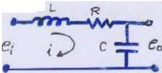
$$L \frac{di}{dt} + Ri + \frac{1}{C} \int idt = e_i \dots \dots (1)$$
