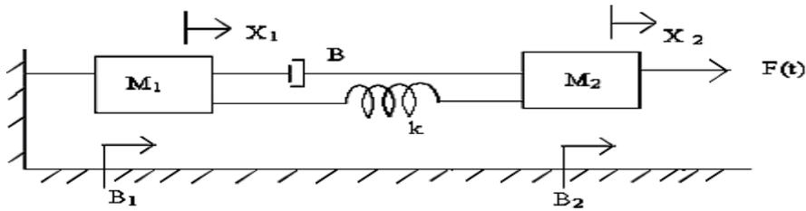
2. Determine the transfer function  $Y_2(S)/F(S)$  of the system shown in fig. (16)
