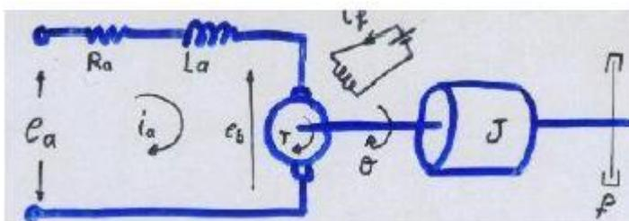
$R_a$  = armature-winding resistance, ohms
