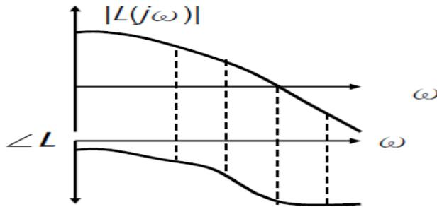
Evaluate  $T(j\omega)$  from  $L(j\omega)$  in the manner of frequency point by frequency point.
