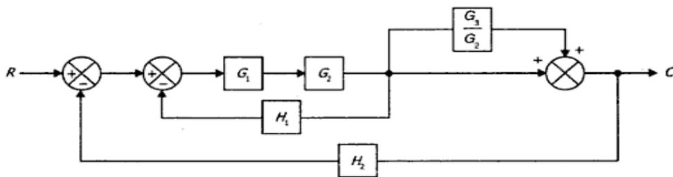
Reducing the cascade block and parallel block
