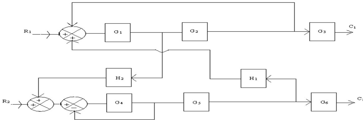
6. Find the overall gain of the system whose signal flow graph is shown in fig. (16)
