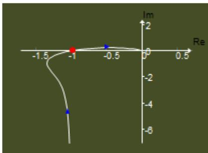
On section bcd,  $s = Re^{j\theta} |_{R \rightarrow \infty}$ ; therefore i.e. section bcd maps onto the origin of the  $G(s)H(s)$ -plane
