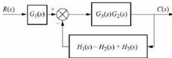
$$\frac{R(s)}{C(s)} = \frac{G_3(s)G_2(s)G_1(s)}{1 + G_3(s)G_2(s)[H_1(s) - H_2(s) + H_3(s)]}$$
