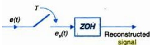
The signal given to the digital controller is a sampled data signal and in turn the controller gives the controller output in digital form. But the system to be controlled needs an analog control signal as input. Therefore the digital output of controllers must be converted into analog form
