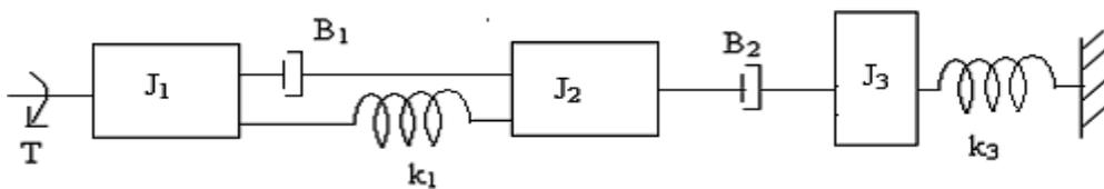
4. Determine the overall transfer function  $C(S)/R(S)$  for the system shown in fig. (16)
