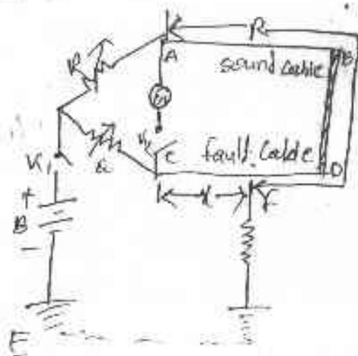
Let  $R$  = resistance of the conductor loop up to the fault from the test end
