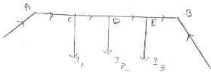
In this type of feeding the distributor is connected to the supply mains at both end & loads are tapped off at different points along the distributor.
