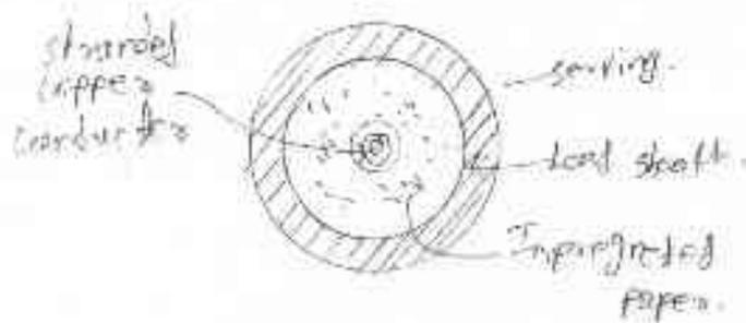
It consists of one circular core of tinned stranded copper insulated by Impregnated paper. The insulation is surrounded by lead sheath. Finally serving is provided over lead sheath to protect the lead sheath from corrosion.
