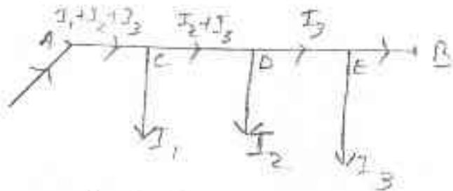
In this type of feeding the distributor is connected to the supply at one end and loads are taken at different points along the length of the distributor.
