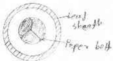
These Cables are used for voltages up to 11 kV.
