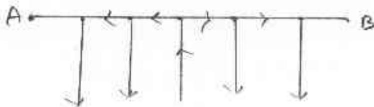
\* In this type of feeding the centre of the distributor is connected to the supply mains.
