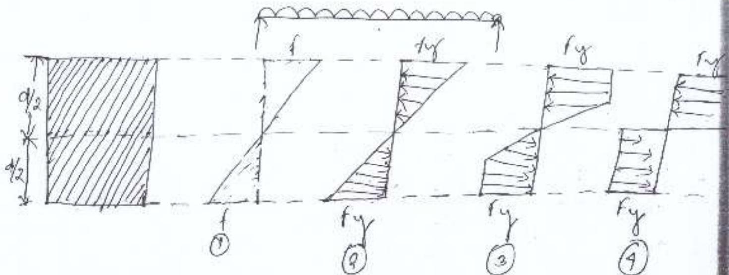
within elastic limit in stage (1), where stress varies linearly from compression to tension.
