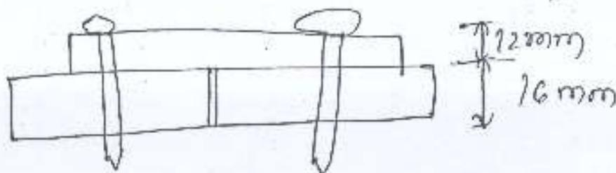
In this case all the bolt will be in single shear and bearing. Strength of the bolt in single shear at the junction of cover plate and main plate.
