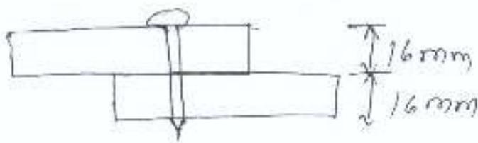
There is only one plane of shearing at the level of two plates, so the bolt will be in single shear & bearing.
