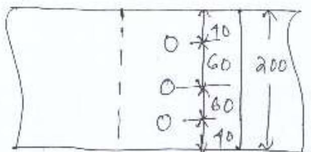
Check for rupture strength of the plate
