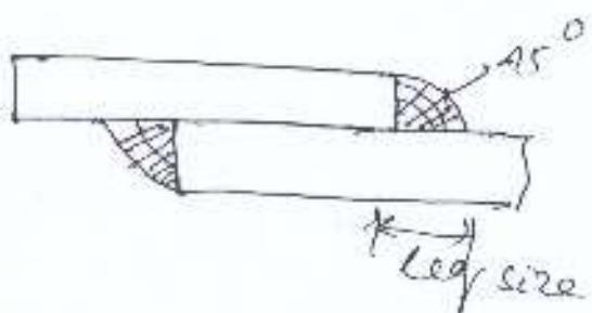
→ When the cross-section of fillet weld is isosceles triangle with face at  $45^\circ$ , it is called as standard fillet weld.
