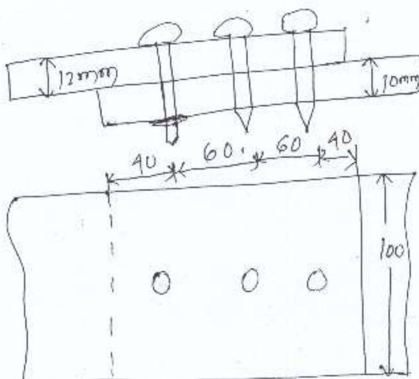
check for rupture strength of the plate
