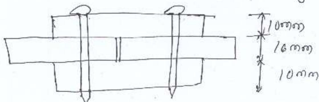
The thickness to be considered for bearing will be the least of the aggregate thickness of cover plates or thickness of the main plate i.e.  $t = 16\text{mm}$
