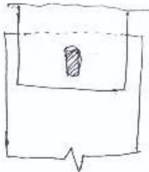
The penetration of these welds into base metal is difficult to ascertain and the inspection of these welds is difficult.
