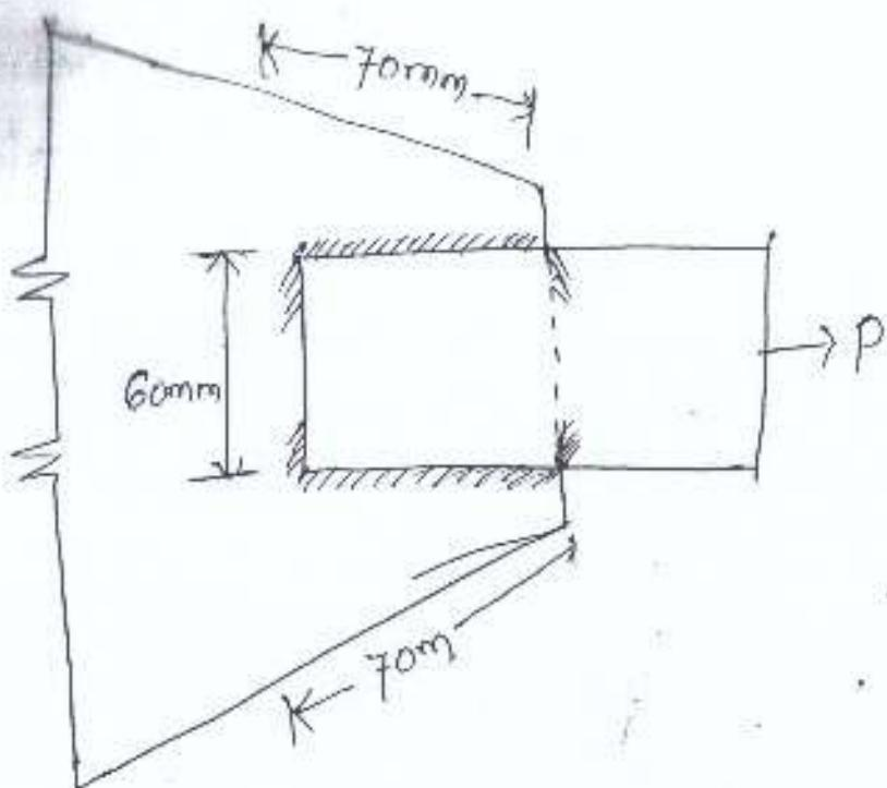
(ii) for field welding on three sides
